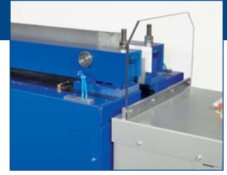
Ergonomic cleaning of the heating element clamping beams
